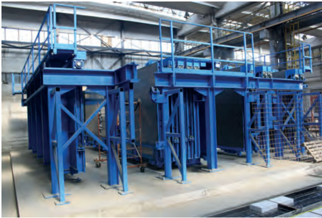
Construx wall battery mould with 10 pockets for the production of the fair-faced double walls
