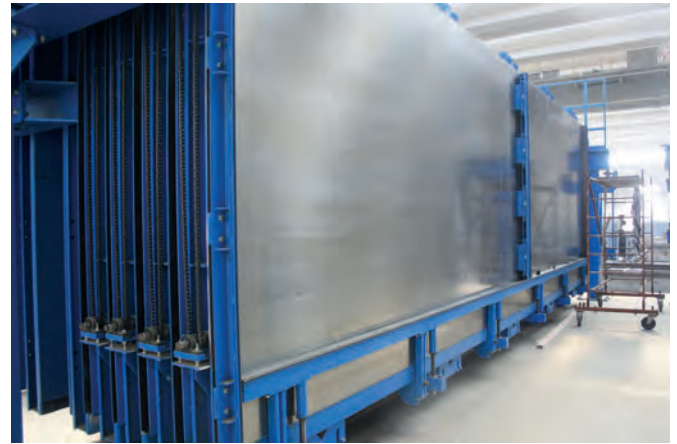
Construx wall battery mould with 10 pockets for the production of the fair-faced double walls
