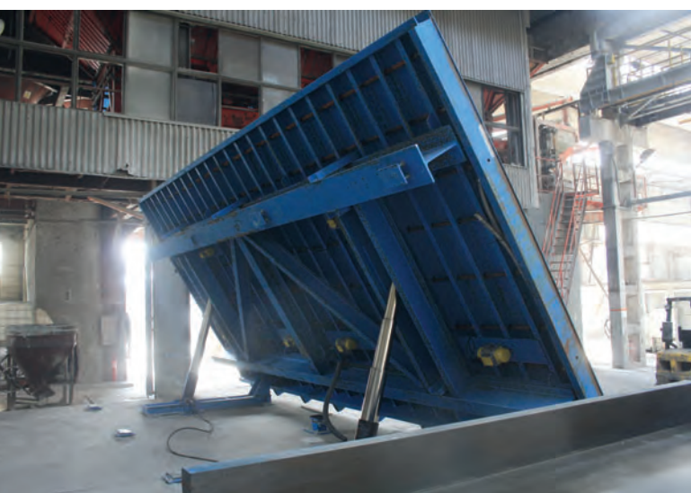
Construx tilting tables (8m x 4m) for the production of the outer walls
